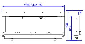
04.TG.3S600 Clear opening = 600mm 04.TG.3S700 Clear opening = 700mm 04.TG.3S800 Clear opening = 800mm 04.TG.3S900 Clear opening = 900mm
